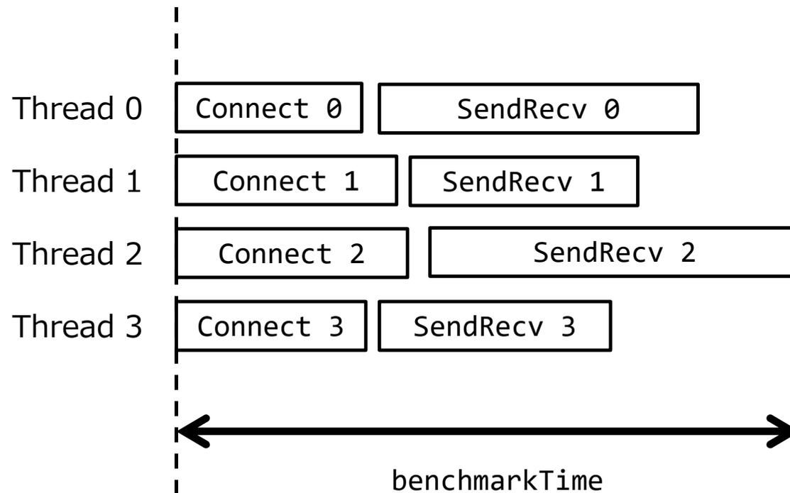
$\text{connectTime}(\text{total}) = \text{Connect } 0 + \text{Connect } 1 + \text{Connect } 2 + \text{Connect } 3$
